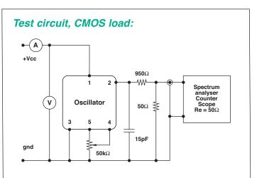
test circuit includes a 20:1 step down into a matched 50 $\Omega$  load
