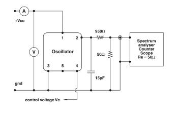
test circuit includes a 20:1 step down into a matched  $50\Omega$  load
